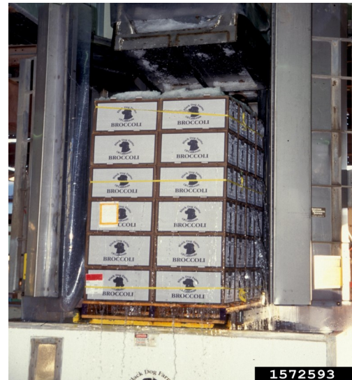
Figure 2. A liquid-icing system for broccoli. Gerald Holmes, California Polytechnic State University at San Luis Obispo, Bugwood.org.
